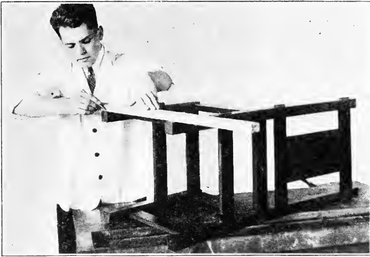
FIG. 401. MARKING CHAIR LEGS FOR LENGTH.
